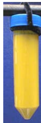
50 mL centrifuge tube containing an aqueous suspension of goethite particles.
